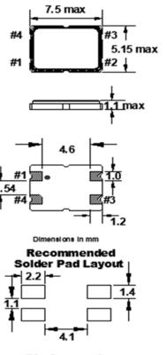
Pin Connections #4 - Lid/Gnd #3 - Crystal #1 - Crystal #2 - Lid/Gnd
