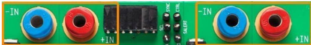
Figure 3.1 Connect 48V between the “-IN” and “+IN” DC power connectors located on the same side of the board (see orangerectangles)
