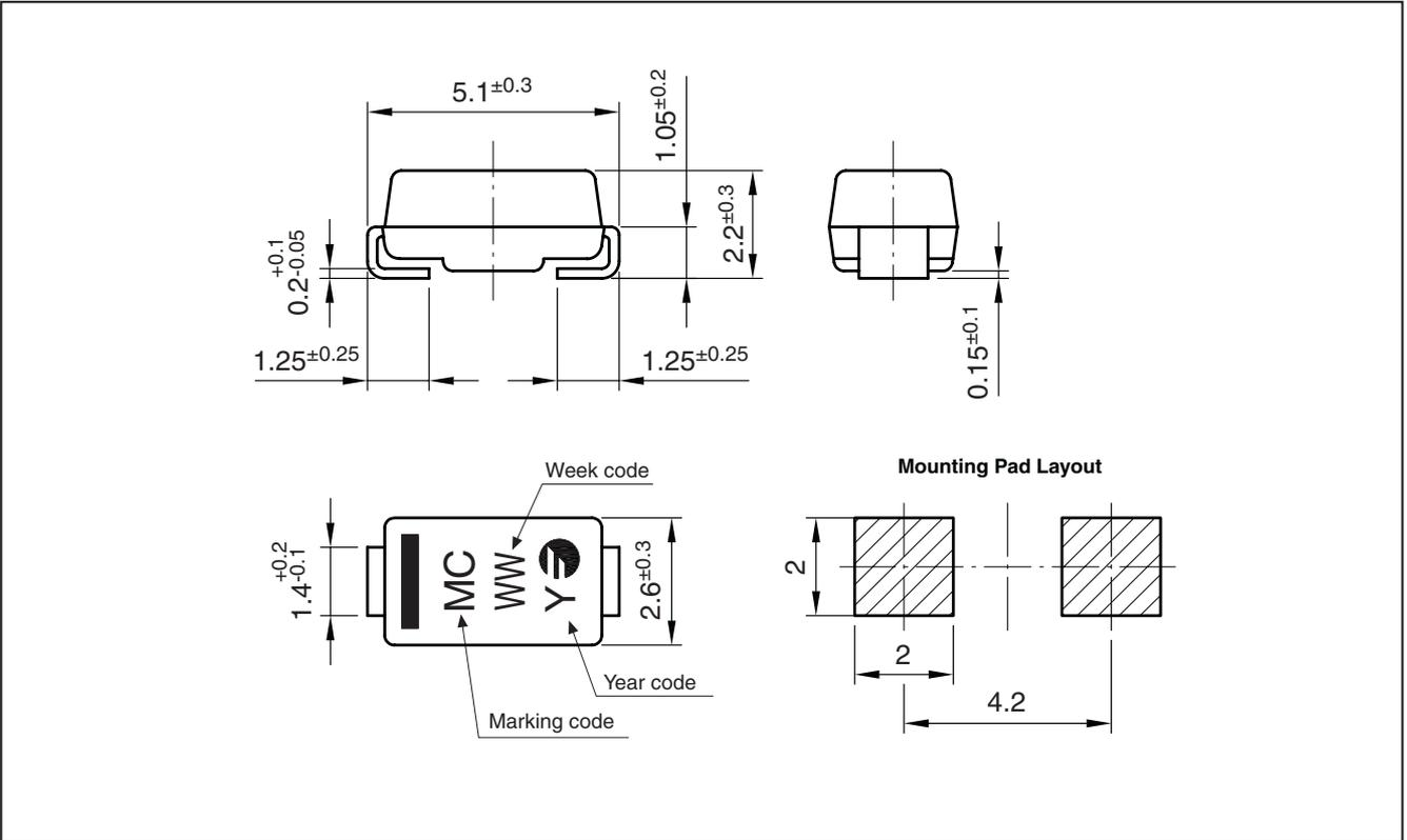
**1.0 Amp. Surface Mounted Glass Passivated Fast Recovery Rectifier**
