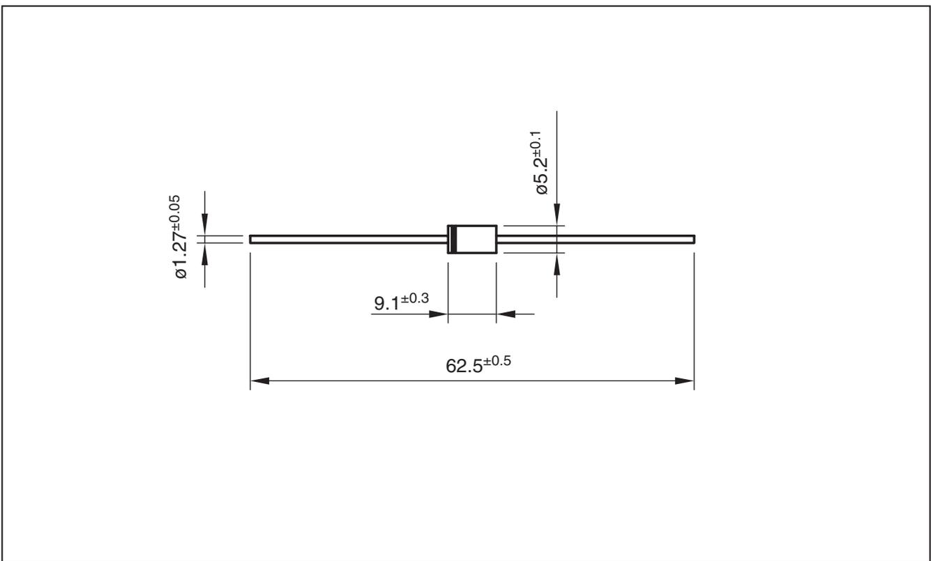
**3.0 Amp. Glass Passivated Junction Rectifier**
