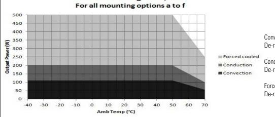
Convection load: 110W up to 50 °C De-rate above 50 °C @ 2.5% per °C
