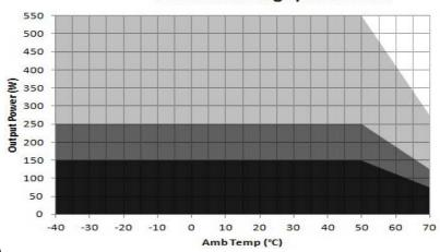
Convection load: 150W up to 50 °C De-rate above 50 °C @ 2.5% per °C
