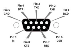
The following table provides the RS-232 signals and their implementations on the Module Assembly. Low-asserted signals have a horizontal line over the pin name.
