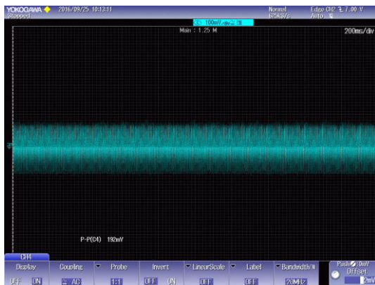
(a) 115V (measured value=190mV)
