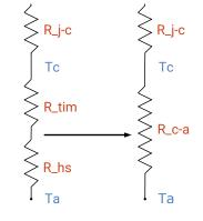
As the figure at right shows, the R\_c-a value is the sum of the thermal resistance of the TIM (R\_tim) plus the thermal resistance of the heat sink (R\_hs).
