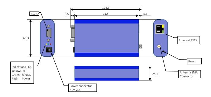
All measurements are in millimeters +/- 0.2mm
