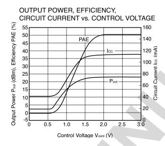
Condition : f = 2,450 MHz, Vcc1 = Vcc2 = Vbias = 3.3 V, Venable = 2.9 V, Vcont = 2.5 V, External input and output matching
