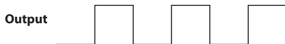
Figure 4: Periodical Output signal could be used to determine the Motor Spinning Speed and Rotation positioning.
