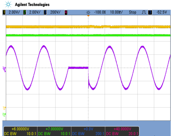
Figure 12 - AC drop out 12ms (10ms/div) CH1: V1 (2V/div) CH2: VSB (2V/div) CH3: Vin (200V/div)
