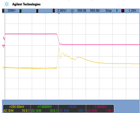
Figure 16 - Load transient V1, 125 to 3 A (500 \mu s/div) CH1: V1 (200 mV/div); CH4: I1 (100 A/div)
