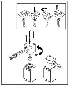
Figure 2. Actuator head may be rotated in 90° increments.
