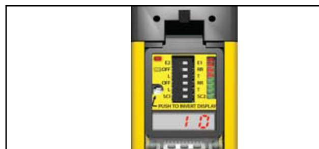
Figure 4-6. Inverted display showing the number 10 and the inverted label
