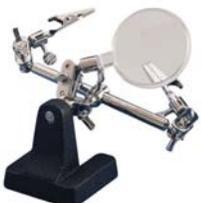
Has an adjustable 2 1/2" diameter magnifying glass. Allows for close observation of work during soldering operation.
