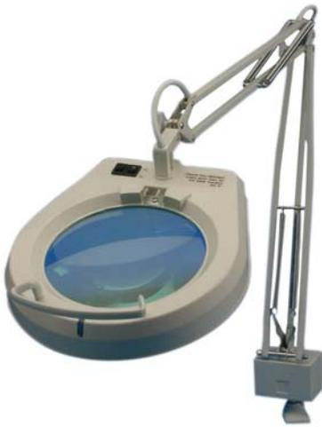
Super large 7", 3-diopter lens gives you unrivaled field of view and work space. Comes with a powerful 32-watt circular fluorescent bulb. This lamp can show you things that you have never seen before! The Ivory mar-resistant engineered plastic housing is mounted on a 45" spring balanced arm for easy positioning. Lamp operates at 115V-AC and comes complete with a mounting clamp and a 5-foot power cord. 1-year warranty (excludes bulb).
