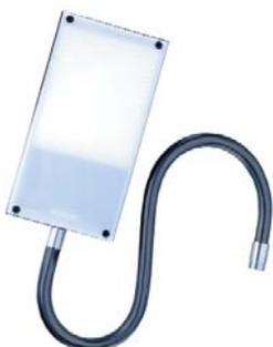
These high-output, uniform backlights are made of the highest quality components and offer a sleek, slim design, which makes them highly versatile for mounting in tight spaces. The housing consists of black, electrocoated steel and the sheathing is PVC covered metal hose. Backlights have a ±10% uniformity. 36" long cable length.
