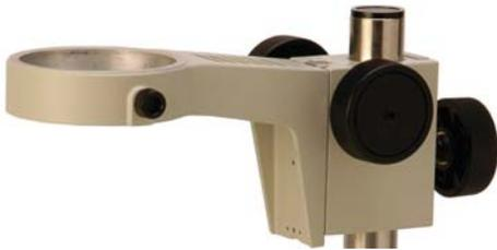
Focus mount to hold our SPZ, DSZ and NSW Series bodies. Rack & Pinion mechanism allows for precise focusing over a 55mm travel. Coarse focus mechanism incorporates a slip clutch and tension adjustment. Fits a 25mm mounting post and has an opening to accept bodies of diameter 74mm (2.9")
