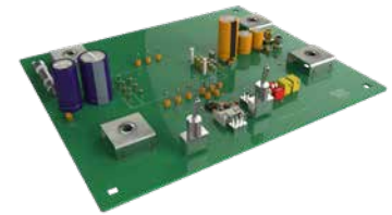
Non-isolated: The demonstration board is populated with two LGA80D modules, allowing you to test independent channel or stacked-module operation.
