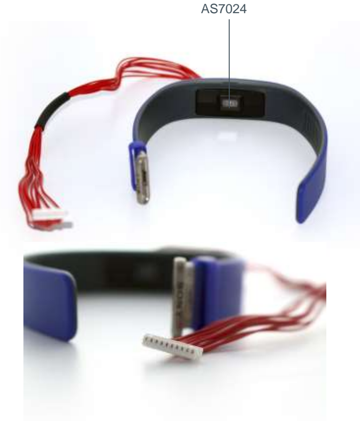
The Wristband also includes the accelerometer (LIS2DH12) and 2 x AS6200
