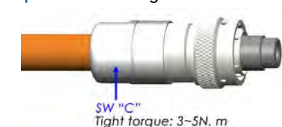
Step 9: Attach and tighten backshell as shown
