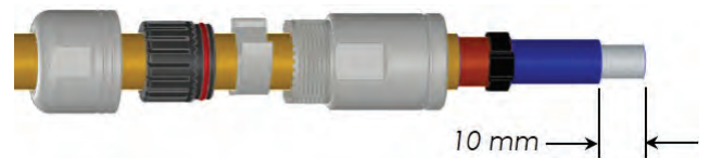
Step 6: Slide plug onto crimped terminal assembly
