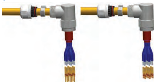
Step 7: Attach contacts to wire leads
