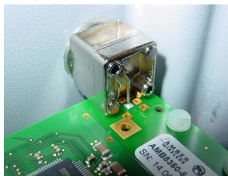
Figure 6 Housing break through with right angled BNC-connector
