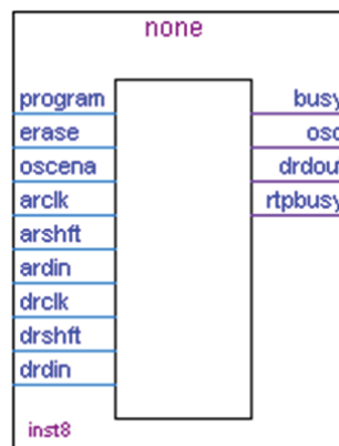
Figure 7-36. ALTUFM_NONE Megafunction Symbol for None Instantiation
