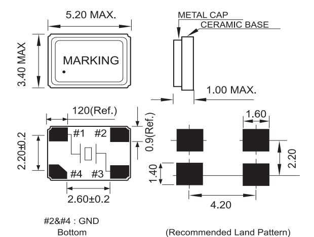
Package is Seam Sealed Ceramic-Metal. Dimensions are millimeters.
