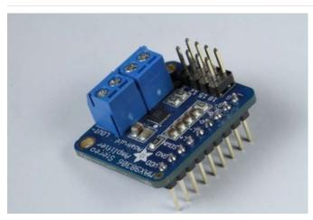
Add Gain Selection and Speaker Terminals Solder the 2x4 pin header for gain selection to the top of the board as shown. Also solder in the 3.5mm screw terminals for the speakers.
