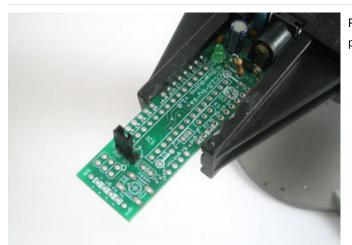
Place the jumper/shunt as shown, so that its on the **EXT** pair of pins.
