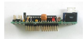
Carefully remove the boarduino by slowly rocking it back and forth to release it from the solderless breadboard.
