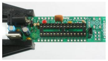
Place the 28 pin socket. This is to allow you to replace the microcontroller if necessary. Make sure the notch in the socket matches the notch in the silkscreened image. In this picture, its on the right.
