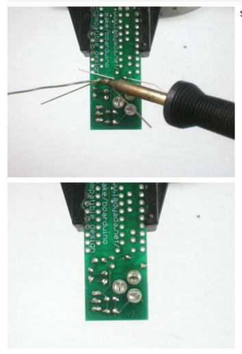
Solder in the resistor and LED and clip the leads.
