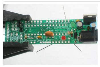
Place the red LED **D3**, taking care to make sure the long lead is in the positive-marked hole. Also place the matching 1K resistor **R3**
