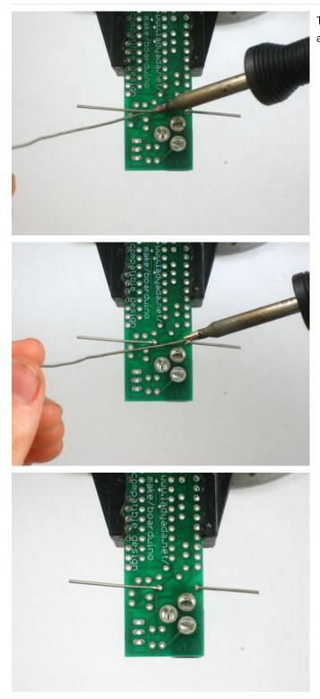
Turn the PCB over and solder both legs so that you get a nice shiny solder joint.
