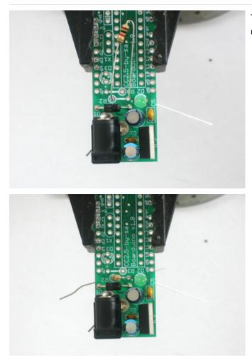
The 1K resistor **R2** goes in, its the LED's matching resistor. Bend it over as shown to place it.
