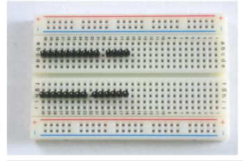
Cut 4 more pieces of header, a 10-pin, 8-pin, 6-pin and 4-pin. Insert them into a solderless breadboard as shown so that the long legs are in the solderless breadboard sockets.
