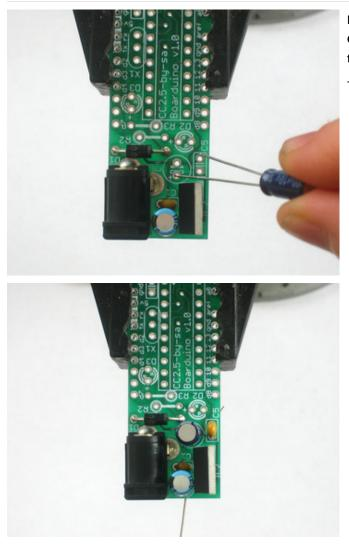
Now you should soder in the 6.3V electrolytic capacitor **C4** as shown. Remember its polarized so you must place the longer lead in the positive-marked hole.
