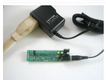
Take the board out of the vise and plug in a power source such as a 9V DC positive-tip wall adapter or a 9V battery with a 2.1mm barrel jack. You should see the green LED light up.
