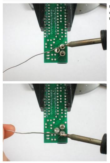
Use the soldering iron to heat up each of the 3 connections and poke the solder in so that it melts into the holes.
