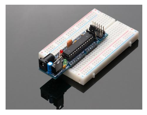
The Boarduino is designed to be inserted into a solderless breadboard, any standard breadboard will be suitable. Simply insert into the breadboard, making sure that the header pins are straight so that they can be easily inserted.
