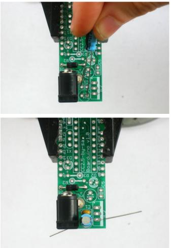
Next, its time to place the 25V electrolytic capacitor **C3**. Electrolytic capacitors are *polarized* which means they only work well in one direction. Put it in backwards and they can explode! You can tell how to place it because the silkscreened image has a plus near one hole and the capacitor has one long lead. That lead is the positive lead. In this image, its the one on the right.
