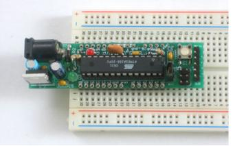
Place the Boarduino on top, so that the header matches up with the solder holes in the PCB.
