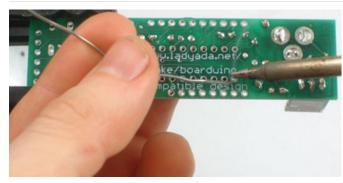
Solder in the socket by tacking two opposite corners and then soldering the rest of the pins. Press the socket into the board to make sure its flat up against it.
