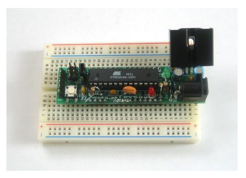
If you are planning to draw a lot of power from the 5V regulator, say for servos or many LEDs, you may want to add a heatsink to the 7805. Just bend the regulator back a bit and slip one on.
