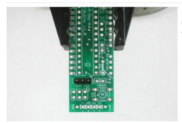
Place the 3 pin header at the other end of the board as shown. the short end goes into the PCB, and the long ends extend up.
