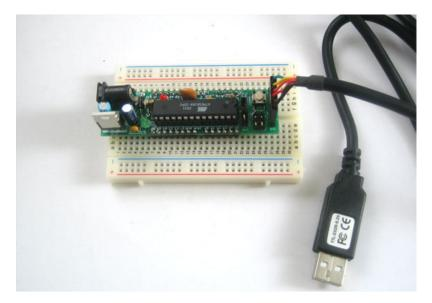
This socket plugs into the Boarduino as shown, and then you can simply plug the USB A connector into your computer. Use the same drivers that you would use with a normal Arduino.
