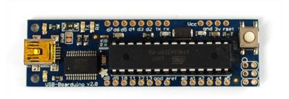
Next, you can attach header pins to make the USB Boarduino fit nicely into a breadboard. If you want to solder wires to the pins instead (free-wiring) you should skip this step.
