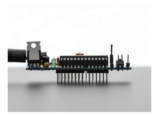
The Boarduino is an Arduino clone: when programmed with the Arduino bootloader, it can talk to the Arduino software and run sketches just like the original.
