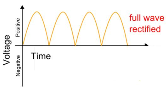
As you can see, there are twice as many humps - there isnt that "half the time, no voltage" thing going on. This means we can divide the calculated capacitor size to half of what it was in the previous.
