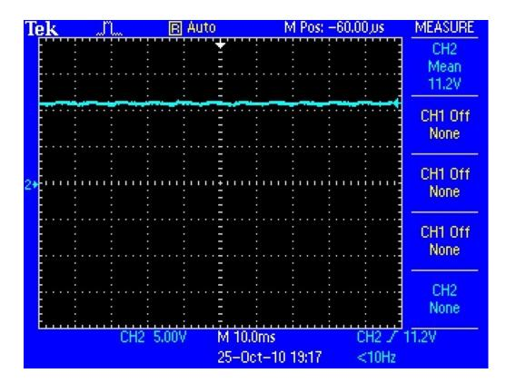
When I connected a 100 ohm resistor (110 mA draw) from the positive pin to the negative pin, it dropped to 11.2V
