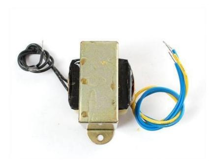
We aren't going to get into the heavy detail of the electromagnetic theory behind transformers except to say that they are made of two coils of wire around a chunk of iron. If the number of coils are the same on both sides then the AC voltage is the same on both sides. If one side has twice the coils, it has twice the voltage. They can be used 'backwards' or 'forwards'! For more detailed information, be sure to check out the wikipedia page (https://adafru.it/alf).
