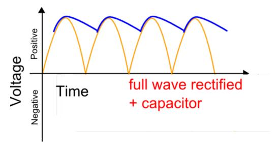
Basically, a full wave rectifier is way better than a half wave! So why even talk about half-wave type rectifiers? Well, because they're useful for a few other purposes. In general, you're unlikely to see an AC/DC converter that uses a half wave as the cost of the diodes makes up for the saving in capacitor size and cost!
