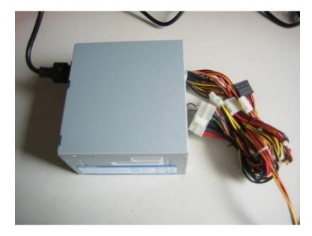
All these power supplies have one thing in common - they take high voltage 120V or 220V AC power and **regulate** or **convert** it down to say 12V or 5V DC. This is important because the electronics inside of a computer, or cell phone, or video game console dont run at 120V and they don't run on AC power!
