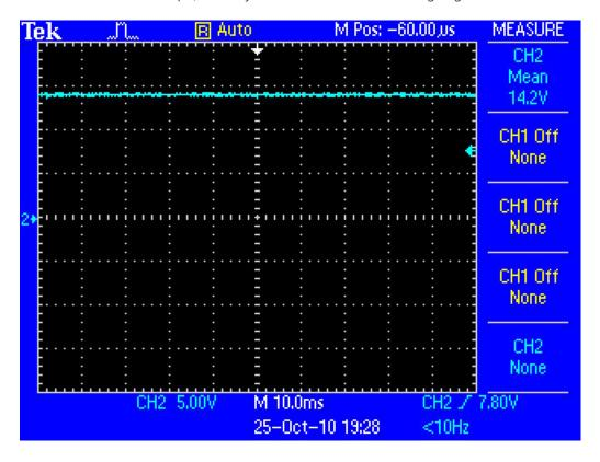
With no current being drawn on the supply, the voltage output is about 14V
