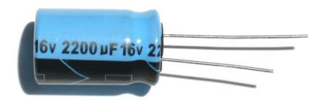
A capacitor **smooths** the voltage out, taking out the lumps, sort of how spring shocks in car or mountain bike reduce the bumpiness of the road. Capacitors are great at this, but the big capacitors that are good at this (electrolytic) can't stand negative voltages - they'll explode!
