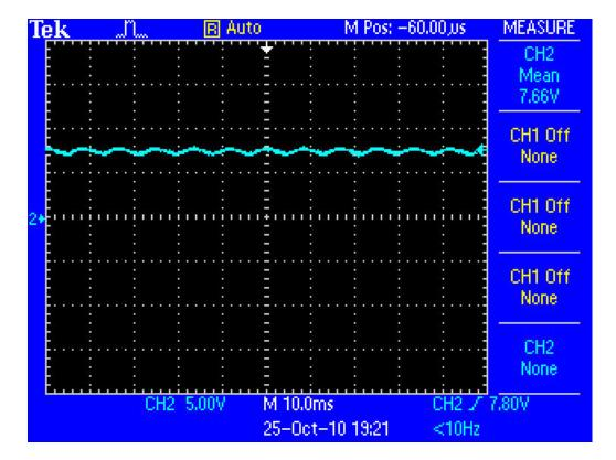
With 35 ohms (230 mA draw) the voltage plummets to 7.7V!
