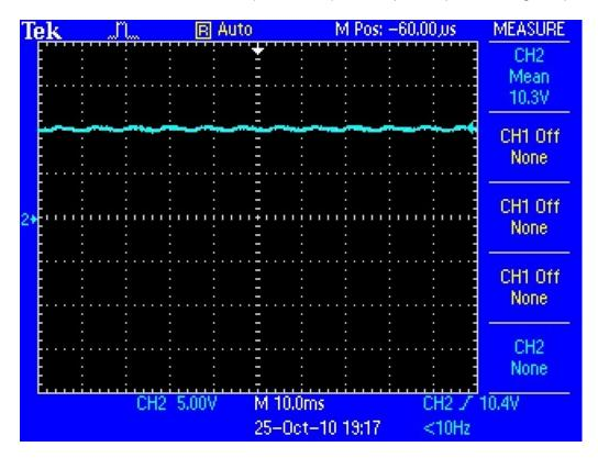
Connecting a 60 ohm resistor (~160 mA draw), it goes down to 10.3V
