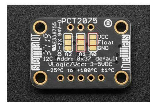
All you need to do is bridge the "Float" pad to either the VCC or GND pad for one or more of the address pins. In the picture above if you bridged the solder pads that are circled, you would pull A0 high to VCC and A1 low to GND. Referring to the table above this would set the address of the breakout to **0x27**
