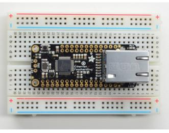
Add the FeatherWing: Place the FeatherWing over the pins so that the short pins poke through the two rows of breakout pads
