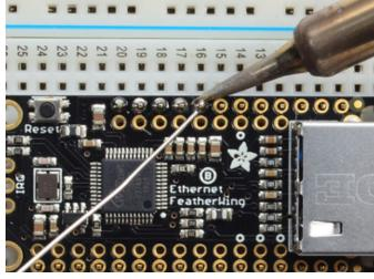
And Solder! Be sure to solder all pins for reliable electrical contact.
