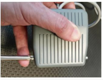
Hold the pedal together with one hand while putting your screwdriver on the metal hinge pin. Keep pressure on the pedal (it is spring loaded) while using pressure to push the hinge pin out.
