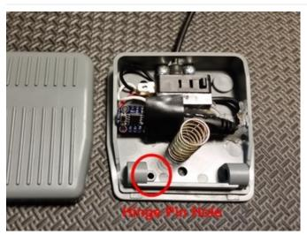
Here you can see the hot glue in place. When replacing the spring, it should not touch the Trinket. To be sure, I used a small piece of electrical tape.
