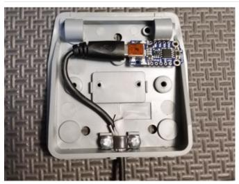
Feed the Mini-B side of the cable through the enlarged hole. Place the Trinket 5V onto the cable end to get a feel for how much cable you want inside the housing (it is a tight fit).
