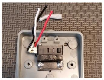
You can carefully grab the grey outer plastic of the short cut cable and slide it off revealing three wires: black, white, and red.
