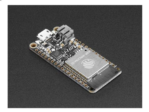
Aww yeah, it's the Feather you have been waiting for! The HUZZAH32 is our ESP32-based Feather, made with the official WROOM32 module. We packed everything you love about Feathers: built in USB-to-Serial converter, automatic bootloader reset, Lithium Ion/Polymer charger, and all the GPIO brought out so you can use it with any of our Feather Wings.
