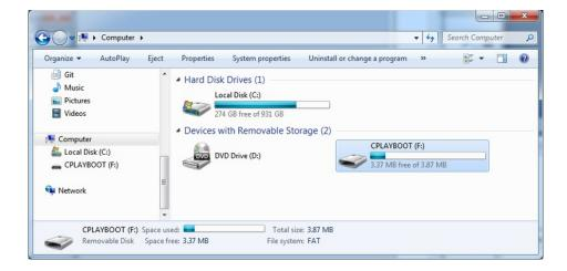
Once the bootloader is successfully connected you can open the drive and browse the virtual filesystem. This isn't the same filesystem as you use with CircuitPython or Arduino. It should have three files:
