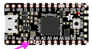
A0 is located between VHI and A1, and the pin pad has left and right white parenthesis markings around it.
