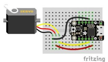
For example, to wire a servo to **Trinket**, connect the ground wire to **GND**, the power wire to **USB**, and the signal wire to **0**.
