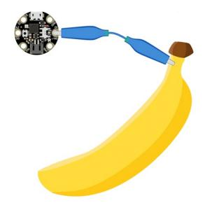
You may need to reload your code or restart your board after changing the attached item because the capacitive touch code "calibrates" based on what it sees when it first starts up. So if you get too many touch responses or not enough, reload your code through the serial console or eject the board and tap the reset button!
