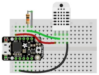
Here's an example using a Trinket M0 - you can use any CircuitPython board, just check that the Data pin is pulseio -capable.
