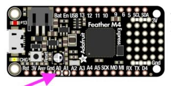
A0 is located between GND and A1 on the opposite side of the board from the battery connector, towards the end with the Reset button, and the pin pad has left and right white parenthesis markings around it
