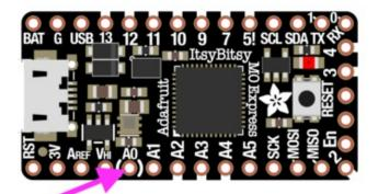
A0 is located between VHI and A1, near the "A" in "Adafruit", and the pin pad has left and right white parenthesis markings around it.
