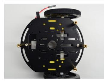
Screw the remaining 2 or 4 standoffs into the second chassis layer.
