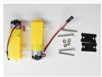
To start, take the two motors, four long screws, four nuts, and two black panels.
