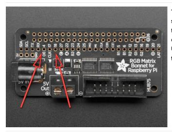
The "quality" option comes at a cost. First, you need to solder a jumper wire between GPIO4 and GPIO18 on the Bonnet or Hat board. Also, the normal sound output of the Raspberry Pi must be disabled. You can still use a USB sound adapter if needed, but audio over HDMI or from the 1/8" jack will not be present.
