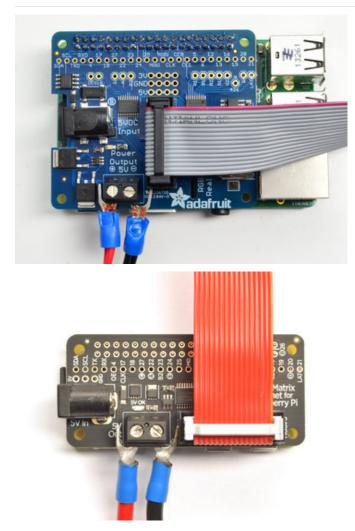
The RGB matrix also came with a 2x8 data cable. Connect one end to the matrix's INPUT side and the other end to the IDC socket on the HAT/bonnet.
