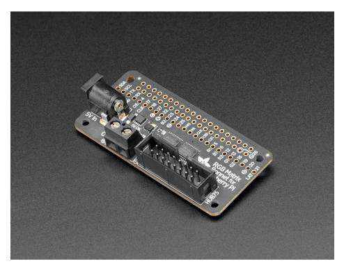
"Bonnet" boards work on any Raspberry Pi with a 40-pin GPIO header — Zero, Zero W/WH, Model A+, B+, Pi 2, 3 and 4. They *do not work* with older 26-pin boards like the original Model A or B. Note with the Pi Zero you may need to
