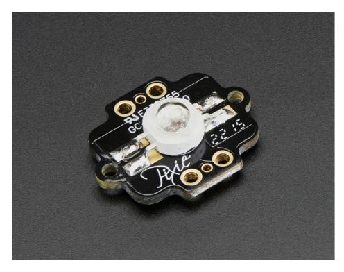
Each Pixie not only contains that aforementioned 3W LED, it also has a Microchip PIC microcontroller. You send it the color you want to appear at standard 115200 baud (1 byte per color). You can send a longer string of pixel data and it will 'forward' along the messages so you can chain them like a shift register. You only have to send the data once per color change. Once set, the microcontroller does all the PWM handling for you.
