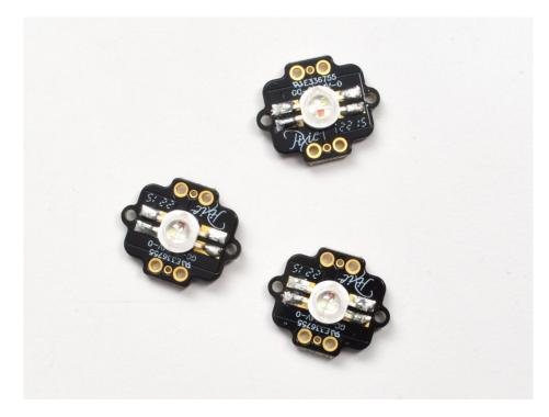
Assembling your Pixies isn't too difficult if you have the right tools and materials. Grab you soldering iron, some thin wire (we like silicone covered 26 AWG) and some thick hefty wire, we used 10AWG stranded.
