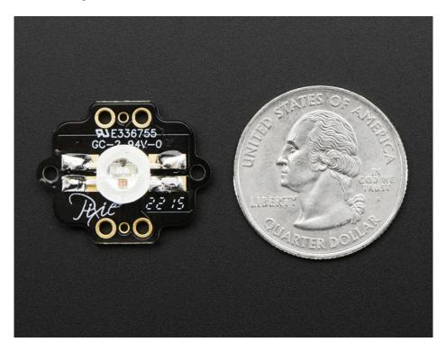
Each Pixie comes fully assembled, with big pads for power wires (don't forget, we're talking about max 1 Amp per Pixie!)
