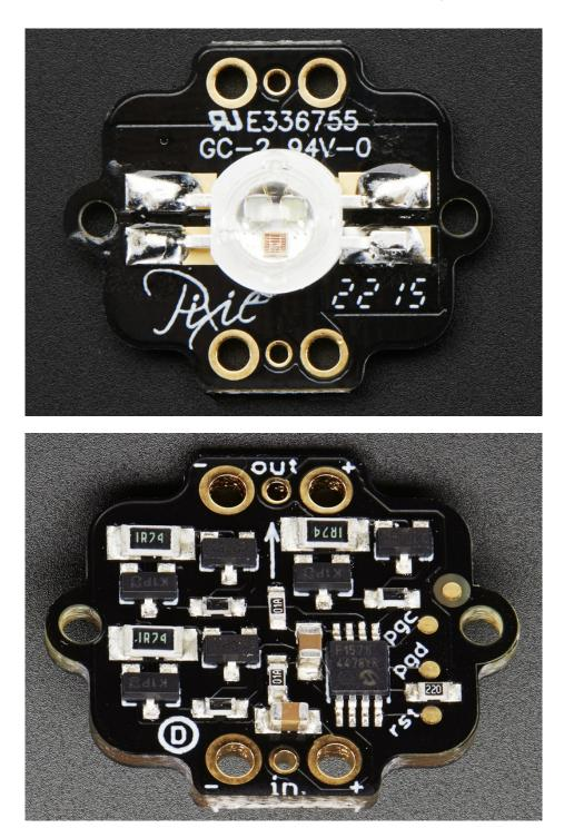
Pixie has two 'ports' - one for input and one for output. Both input and output ports have power pins:
