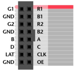
**Either end of the ribbon cable can be plugged into the matrix INPUT socket.** Notice below, the "key" faces the same way regardless.
