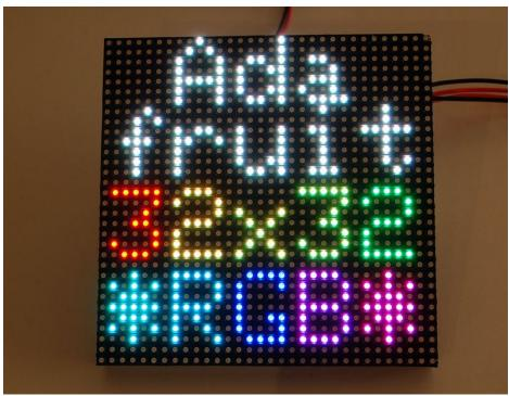
These panels require 12 or 13 digital pins (6 bit data, 6 or 7 bit control) and a good 5V power supply, at least a couple amps per panel. We suggest our 2A (or larger) regulated 5V adapters and either a terminal block DC jack, or solder a jack from our DC extension cord. Please read the rest of our tutorial for more details!
