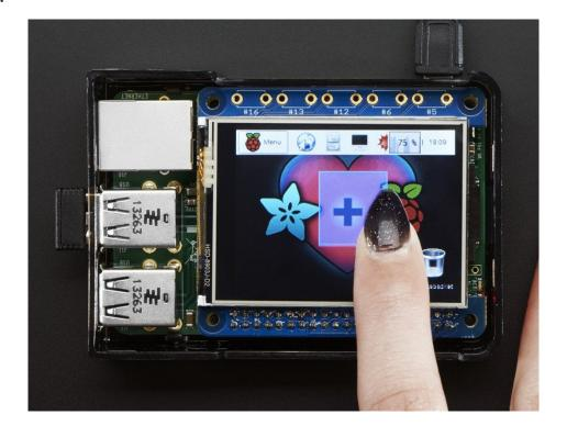
Is this not the cutest little display for the Raspberry Pi? It features a 2.4" display with 320x240 16-bit color pixels and a resistive touch overlay. The HAT uses the high speed SPI interface on the Pi and can use the mini display as a console, X window port, displaying images or video etc. Best of all it plugs right in on top!
