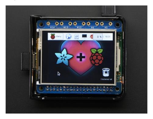
This design uses the hardware SPI pins (SCK, MOSI, MISO, CE0, CE1) as well as GPIO #25 and #24. All other GPIO are unused. Since we had a tiny bit of space, there's 5 spots for optional slim tactile switches wired to five GPIOs, that you can use if you want to make a basic user interface. For example, you can use one as a power on/off button.
