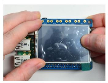
Line up the TFT screen so it matches the white outline and press it down to stick it to the circuit board
