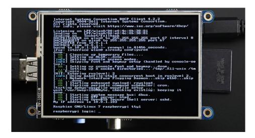
One fun thing you can do with the display is have it as your main console instead of the HDMI/TV output. Even though it is small, with a good font you can get 20 x 40 of text. For more details, check out https://github.com/notro/fbtft/wiki/Boot-console (https://adafru.it/cXQ)
