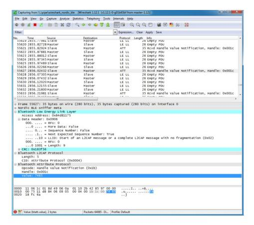
The results of this transaction in the nRF UART application can be seen below:
