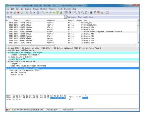
What this write request is trying to do is enable the 'notify' bit on the UART service's TX
