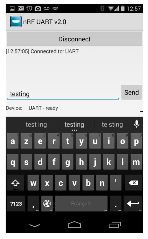
On the BLEFriend side we can see the 'testing' string that was sent from nRF UART in the terminal emulator below:
