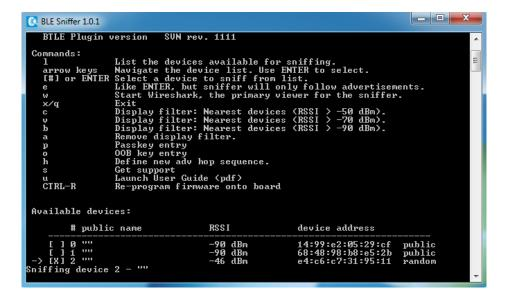
At this point you can type 'w', which will try to open wireshark and start pushing data out via a dedicate pipe created by the nRF-Sniffer utility.
