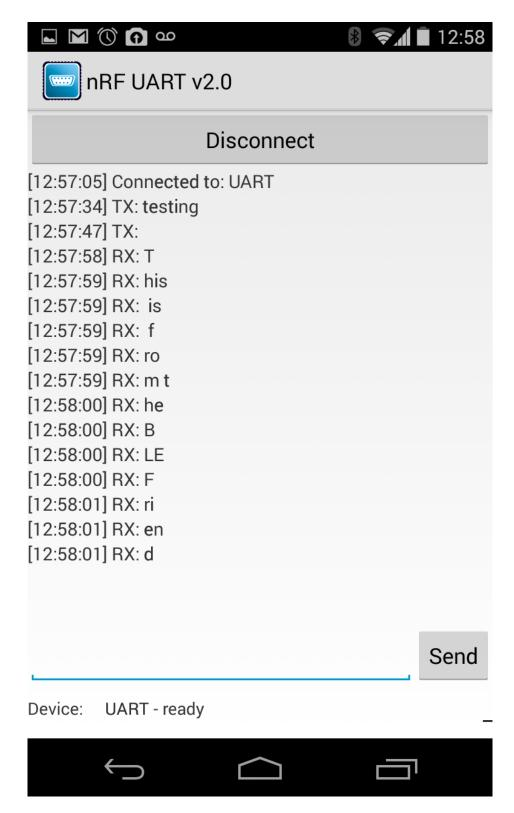
The incoming data is broken up into small packets because it is transferred in chunks of up to 20 bytes per payload.
