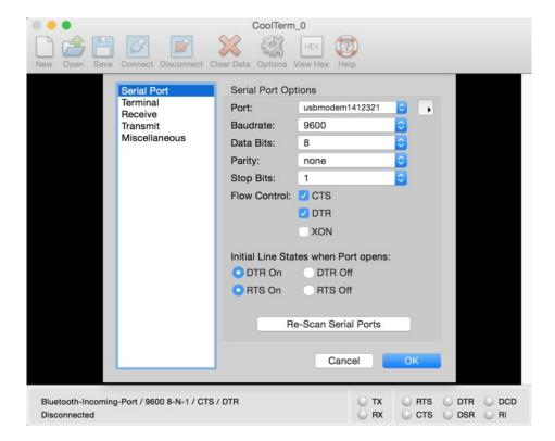
Make sure you click the 'Connect' button to open the connection in CoolTerm, and 'Disconnect' to close the connection when you are done.
