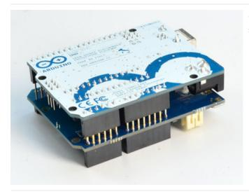
Check your work by looking to make sure the pins are soldered
