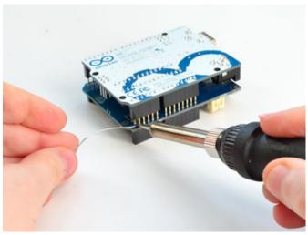
Tack the outer pins of each stacking header. This way they'll be aligned right.
