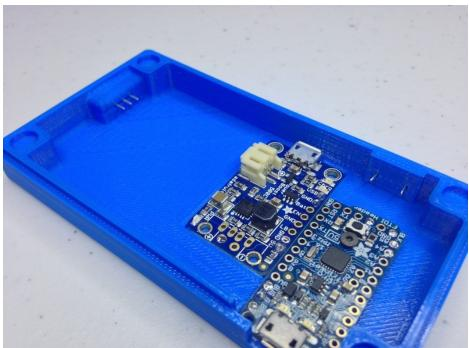
Push the SPDT switch into the cavity at the top of the enclosure, and the pushbutton on the right side of the enclosure. You should be able to see the pins of the switch and pushbutton on the inside of the enclosure.
