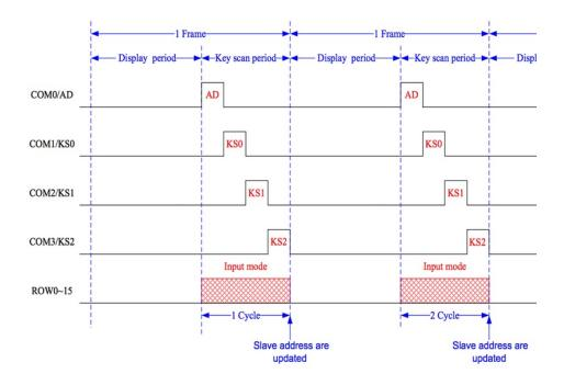
The HT16K33 refreshes the LED matrix with a frequency of about 100Hz. In each of the 10ms frame, it first refreshes the display, and then scans the button matrix for the state of every single one of those 13x3=39 buttons. But it's gets
