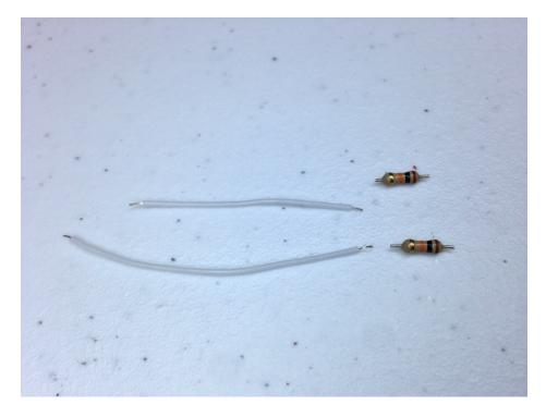
Now prepare two resistors and two short piece of wires - approximately 4cm and 5cm respectively - and solder each wire to a resistor.
