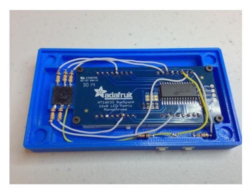
Then we can solder the last set of wires to connect the two resistors on the right side of the joystick to the backpack. Again, please refer to the circuit diagram on the previous page if the picture looks confusing.
