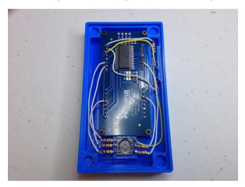
Now we have the top half of the Tiny Tetris with all components assembled and wires soldered.
