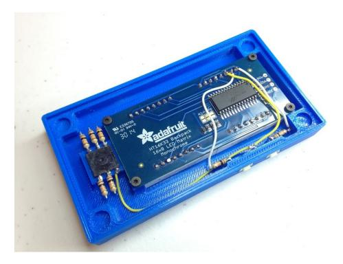
Solder the two white wires from the pushbutton resistors to the 1st and 2nd pins on the left side of the top LED matrix.
