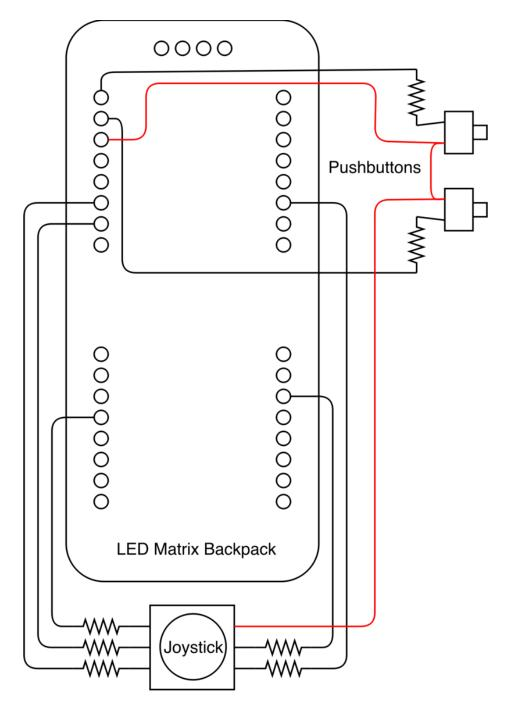
The second circuit diagram contains everything mounted on the top half of the enclosure. This is a view from the inside of the enclosure, which means that both the LED Matrix Backpack and the joystick are facing away from us. If it seems confusing, the assembly guide on the next page will definitely help you understand better. All seven resistors shown in this circuit diagram have a value of  $10k\Omega$ .
