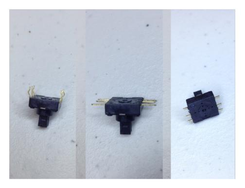
To prepare the joystick for soldering/mounting, straighten its legs, bend them 90 degrees outward, and then cut them to about half the length.
