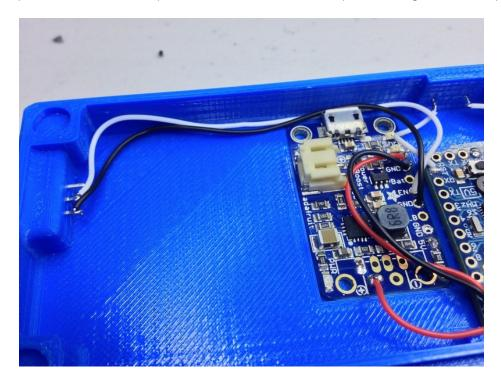
Now connect the EN and GND pins on the PowerBoost to the left and middle pins on the SPDT switch. Be sure to run the wires on the side instead of going straight to the switch. We want to leave some space for the LiPo battery.
