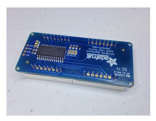
Let's start with the soldering the LED matrices to the Backpack. After all 32 pins have been soldered, carefully trim the pins with a flush cutter.
