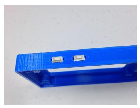
Be careful when soldering inside the enclosure. Your soldering iron will deform the PLA plastic if they come in contact with each other (see the burn mark in the picture below.)
