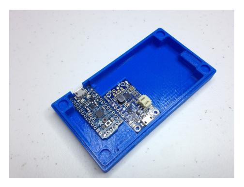
Start by putting the Pro Trinket and the PowerBoost 500 Charger into the enclosure. Use a M2 screw to secure the Pro Trinket. Gently push the PowerBoost into the cavity to fix it in place. It should be more or less a friction fit.
