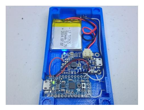
Finally we can connect the battery to the JST connector on the PowerBoost to test the circuit. If you slide the SPDT switch to the right, the boost converter will be enabled, and the system will power on. Make sure that you see both the blue LED on the PowerBoost and the green LED on the Pro Trinket light up.
