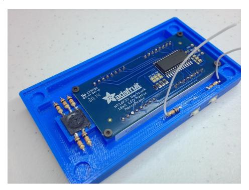
Now push the LED matrix backpack into the largest opening, and use four M2 screws to secure it in place. Make sure that the I2C pins (VCC, GND, SCL, SDA) are near the top of the device.
