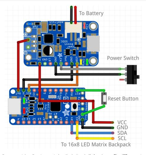
This first circuit diagram contains all parts mounted on the bottom half of enclosure. The JST connector on the PowerBoost 500 Charger goes to the LiPo battery, which is not shown in the picture. The four wires that connect to the 16x8 LED Matrix Backpack are the only ones that connect between the bottom and top half of the enclosure.
