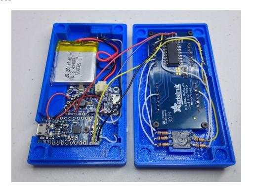
Connect the four wires to the Pro Trinket and PowerBoost as listed below:
