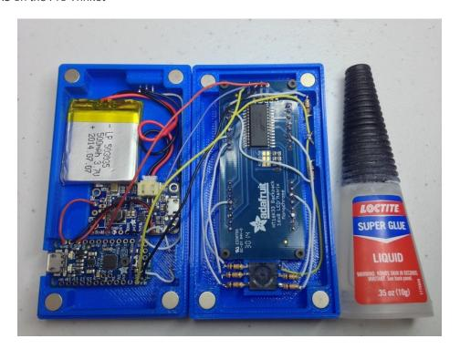
Finally use some super glue to secure the eight magnets to the cavities on the enclosure. Wait for a little bit to allow the glue to dry completely.
