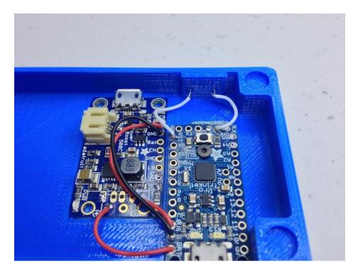
Then use two more short wires to connect the reset button to the Pro Trinket.
