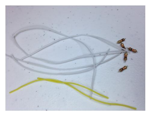
Prepare 5 pairs of resistors and short wires (about 8cm each). We'll cut them to the exact lengths needed later.
