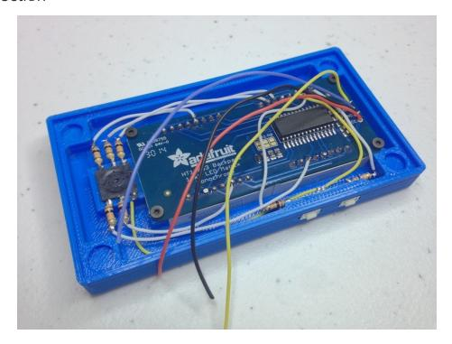
Solder four wires to the I2C pins on the Backpack. The colors I used in the picture above are the same as the ones in the circuit diagram on the previous page.
