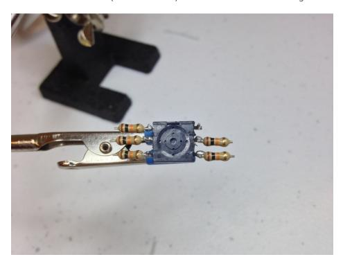
Solder the five resistors to the five pins on the joystick. Make sure the solder makes firm connections between the resistors and the joystick.
