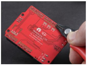
Trim the pins on the back and you are ready for the final assembly of your Pixy Pet!
