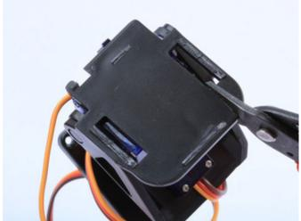
Cut a notch for the cable connectors We need to make room for the cable connectors on the back of the camera module. Two cuts, as shown in the photos will remove the top left side of the bracket.
