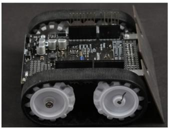
Plug the headers upside-down into the Zumo Chassis as shown.
