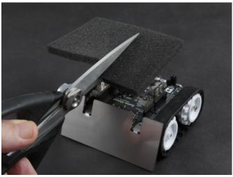
Using a piece of the packing foam from the Seeeduino kit, cut two small squares roughly 1.5"x1.5" (3.5cm x 3.5cm) - These dimensions are not super critical!
