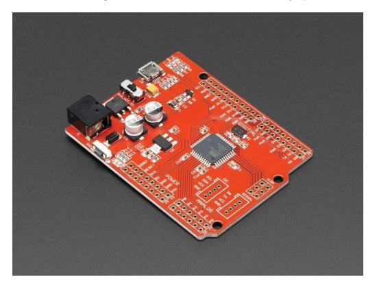
There is one little problem though. The Zumo chassis has a couple of unfortunately placed capacitors that interfere with the DC jack and capacitors on the Seeeduino. The good news is that the Seeeduino ships without headers installed. So all you need to do is replace them with slightly longer headers. The Arduino R3 Stacking Headers (http://adafru.it/85) are just the thing we need.
