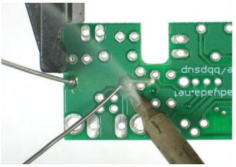
Now solder both wires to the PCB.
