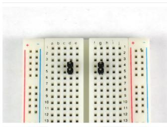
If your breadboard has nonstandard spacing, you can still plug it in using the header-breakouts in the middle.
