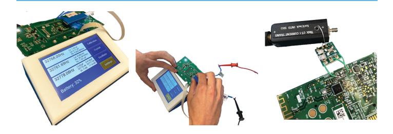
Historically, design engineers have optimized their circuit performance via trial and error, at the expense of significant investment in time. Further, to properly determine the oscillator loop dynamics, there is no other choice but to break the oscillator loop and make key measurements using specialized equipment such as a current probe.
